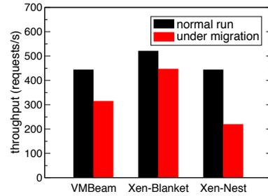
Figure 7. The degradation of web performance under VM migration.
